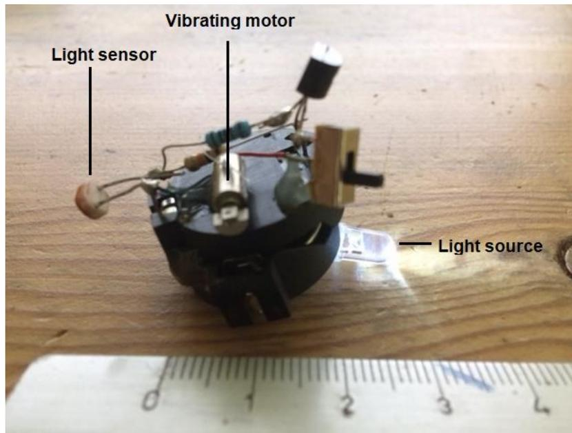
*Robot with a sensor and a source.*
